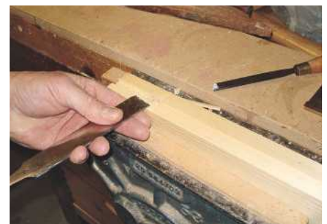
▲ Pic.21 ...a flat area ready to receive the square shoulder of the rail
